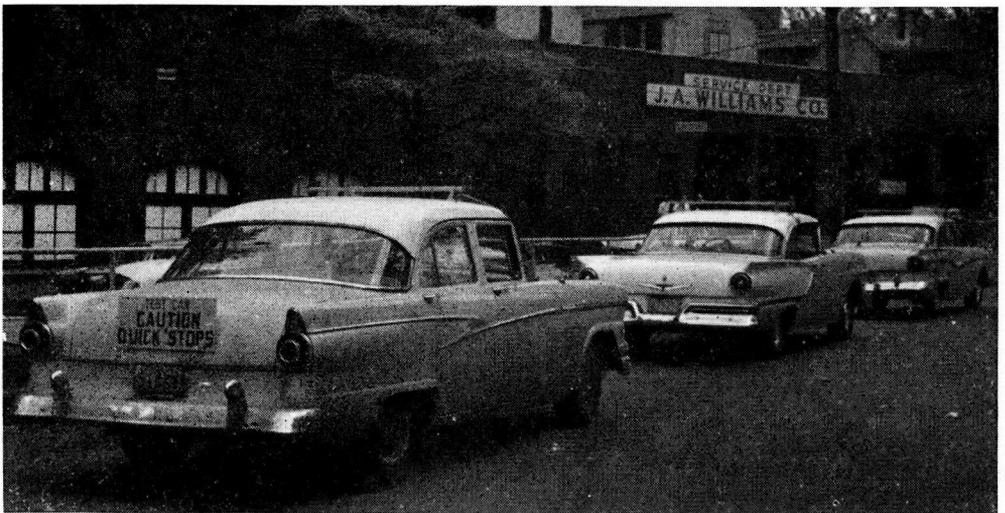
Plate B. Experimental platoons showing marker lights on roof racks.
