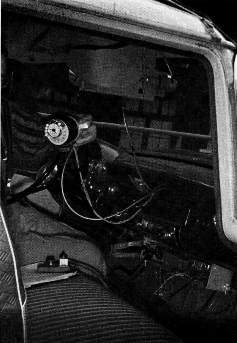
Plate A. Recording equipment and camera mounted in car showing indicator lights on speedometer dial of camera.
